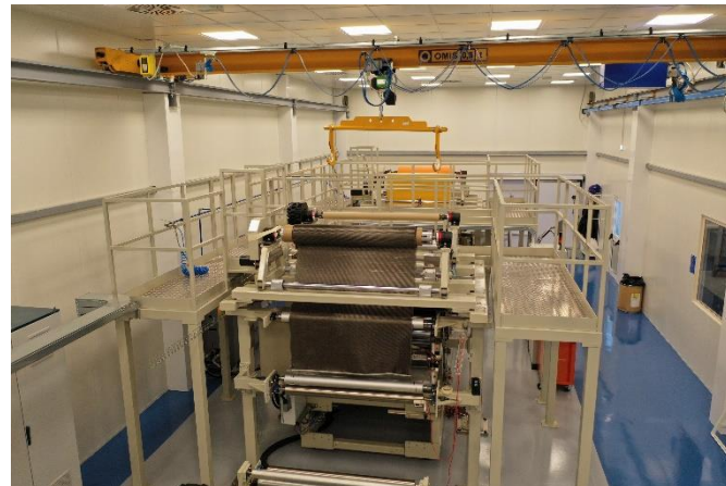
Hot-melt prepreg line for prepreg manufacturing at Nano Tech
