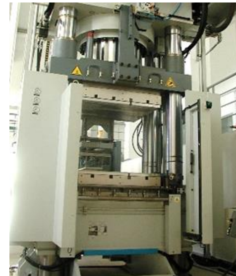
Pilot-scale (CETMA) press for PCM process development
