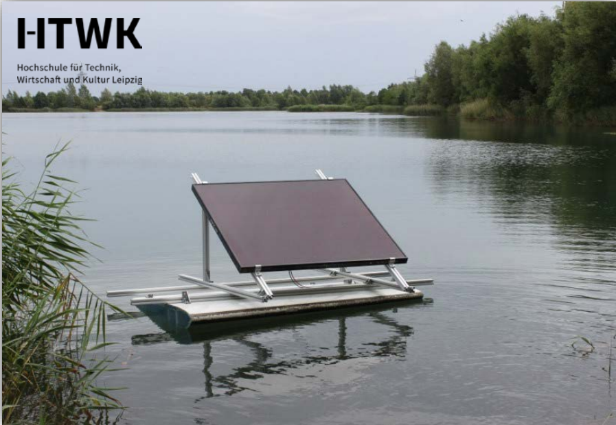
Float test with PV-floating system
