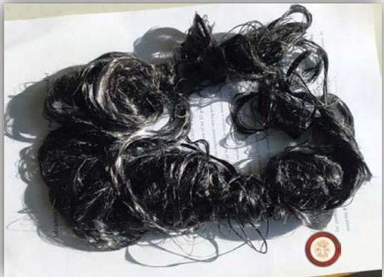
Continuous Carbon Fibre Reclamation through Plasma Treatment
