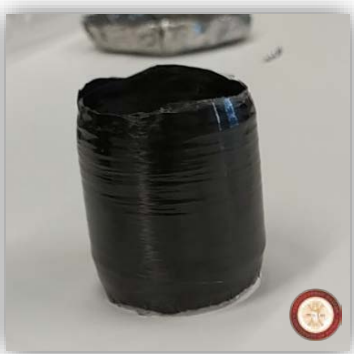
Composite specimen manufactured with Filament Winding
