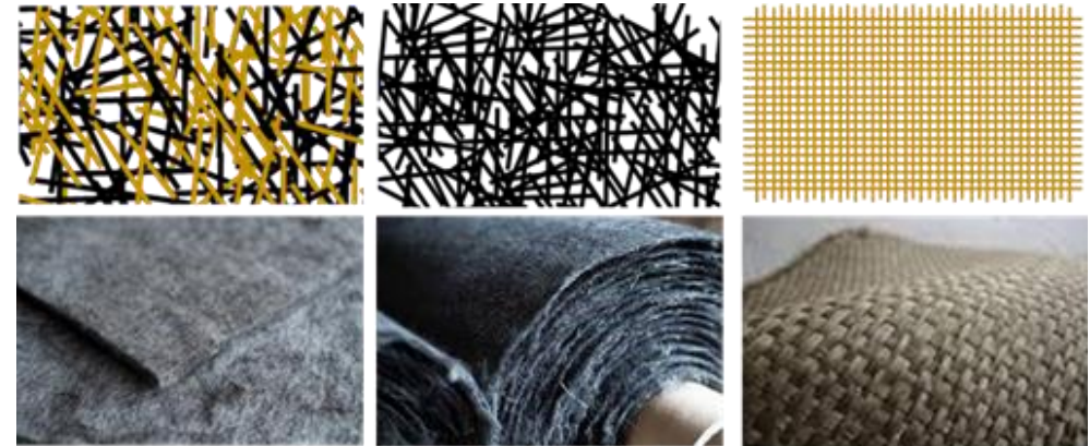
Fiber architectures at ply level - (a) innovative hybrid commingled hemp/ rCF non-woven, (b) commercial rCF non-woven, (c) hemp fabric
