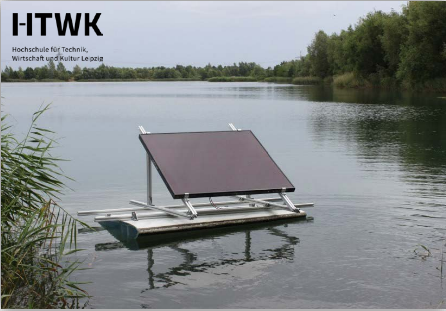
Float test with PV-floating system
